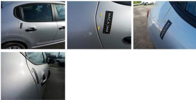
Porte ARG, Griffe(s), Acceptable
